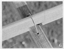
and exhibits a good snug fit (but not too tight), drill a hole through the deck beams about 2.5 centimeters inboard of the gunwale and lash the joints together as shown in photograph B. File notches to recess the lashings. Thin, braided nylon cord, such as mason's twine or fisherman's net twine, will do well. Take about four or five tight wraps at every joint.
