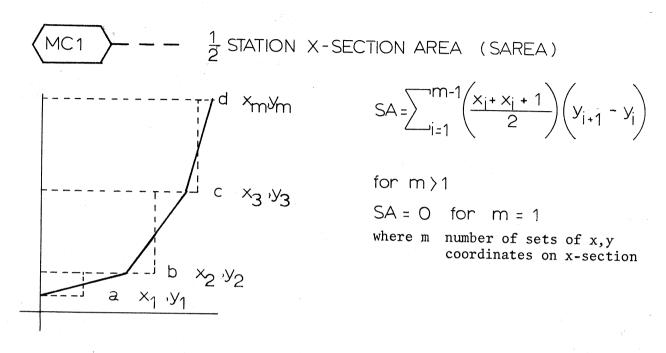
Where hull is rounded and not multi-chined, greatest accuracy is obtained using as many sets of x,y coordinates as possible (up to 9 sets allowed)
