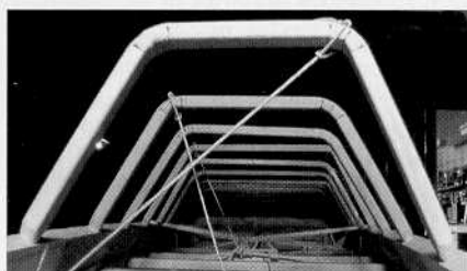
As the ribs are set into the gunwales they must be tuned to keep them flat across the middle and parallel with each other.
