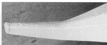
The center seam is sewn from the ends toward the cockpit.
