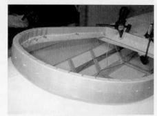
The canvas is pinned to the inside of the coaming with the edge folded under. A clamp holds the aft end of the coaming in place on the itivik.
