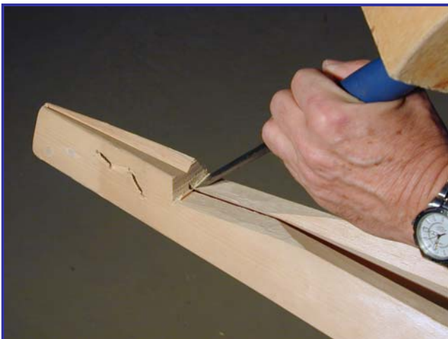
Figure 58. 29-3 Bow showing keelson inlet into the gunwales.
