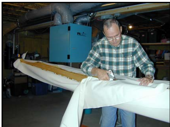
Figure 79. Cutting the canvas to fit.
