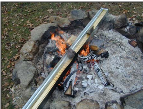
Figure 26. Boiling the wood in a converted eaves trough with ends capped.
