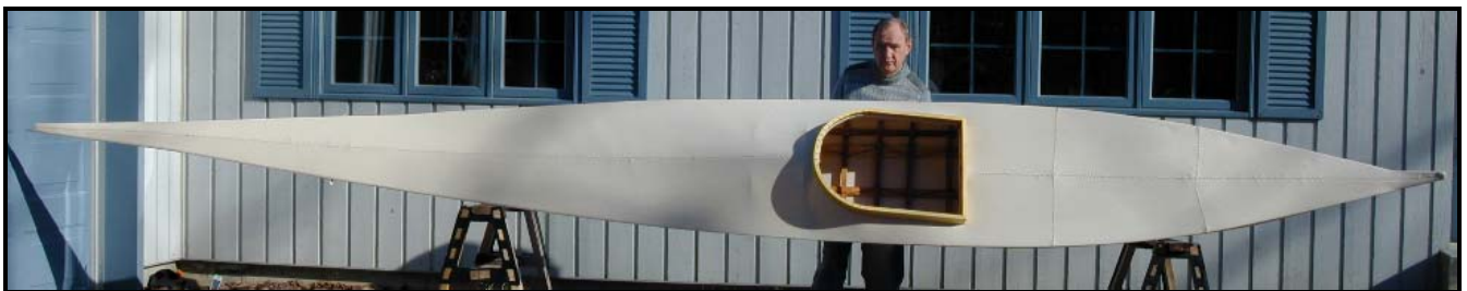
Figure 100. Kayak with canvas and one coat of dope – plan view.
