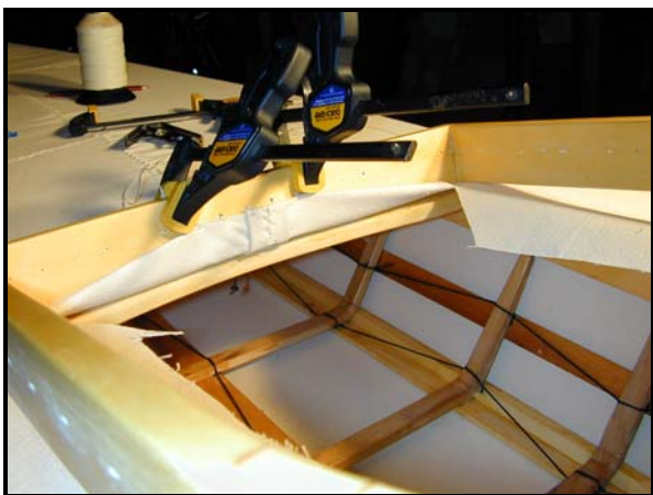
Figure 90. Fitting canvas to coaming.
