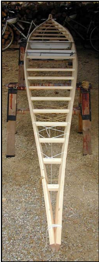
Figure 29. Kayak gunwale, deck beams, temporary masik and itivik from front view.
