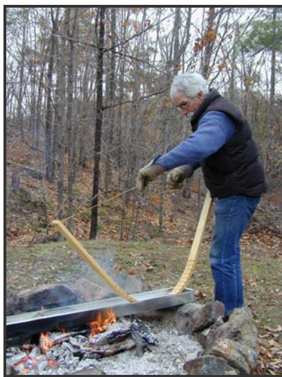
Figure 27. A boiling container is made from a length of eaves trough with the ends capped.
