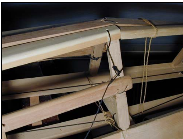
Figure 64. Bilge stringer tied on at bow.
