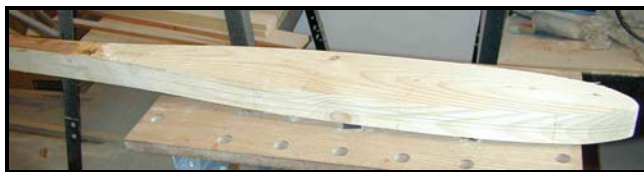
Figure 109. First shaping planed/smoothed on the plan view.
