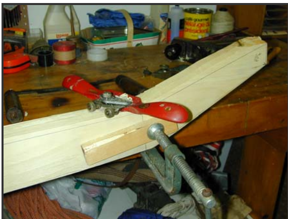
Figure 6. Using spokeshave to shape stern handhold.
