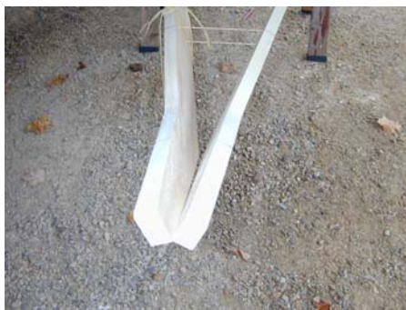
Figure 19. Closeup of bow with holes through gunwales for lashing.
