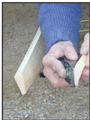
Figure 22. Gunwales spread apart for planning bow.
