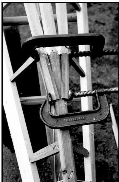
Figure 69. Fairing blocks for bow area bilge stringers.
