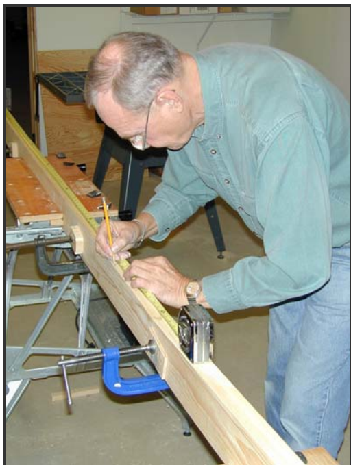
Figure 11. Marking the deck beams on the gunwales.
