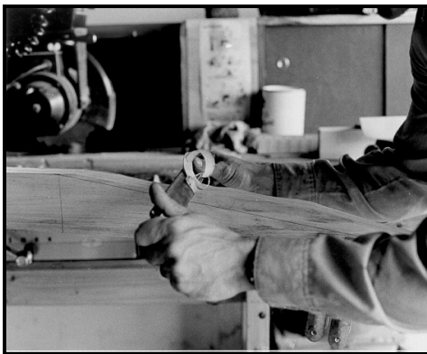
Figure 4. Gunwale with drawknife cutting away scarf joint.
