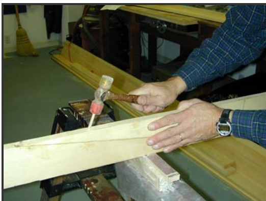
Figure 9. Driving in a wooden peg in gunwale scarf joint.
