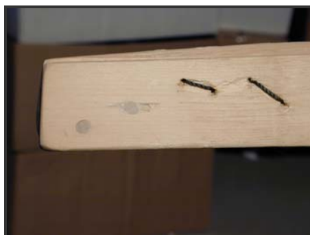
Figure 23. Bow side view with sewing and dowels. Figure 24. Stern bottom view with dowels.
