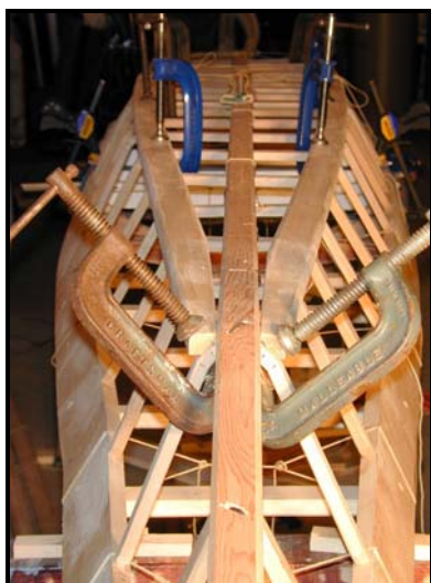
Figure 63. Keelson lashed in place.
