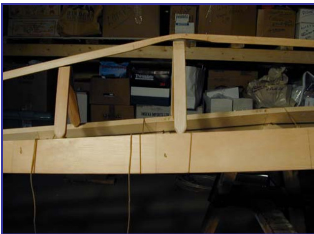
Figure 55. Keelson planed thin at bend in stem.
