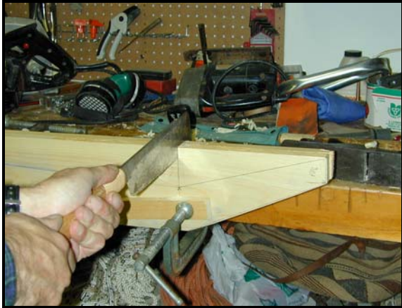
Figure 2. Sawing the stern handhold.
