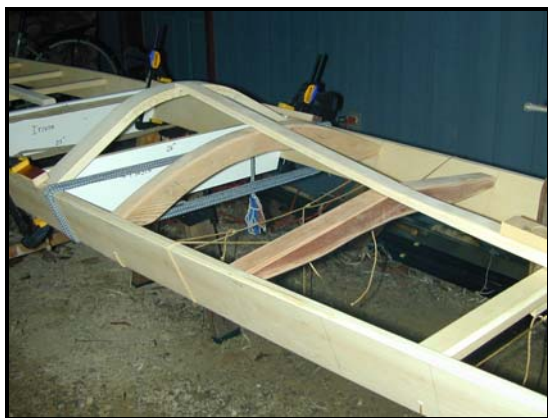
Figure 38. Masik and two forward deck beams.
