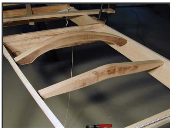
Figure 28. Masirusigiik (two small deck beams)
