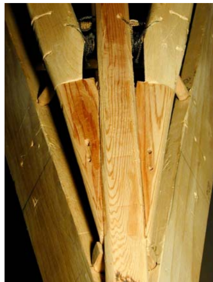
Figure 66. Glued in fairing pieces on stern of bilge stringer.
