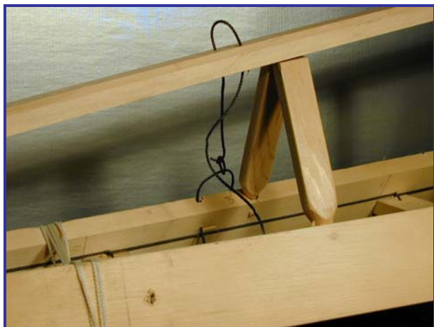
Figure 61. Loosely-tied gunwale/keelson lashing.
