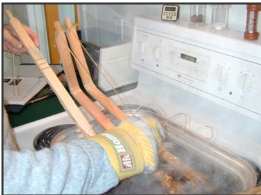
Figure 49. Ribs boiling in water to heat them for bending.
