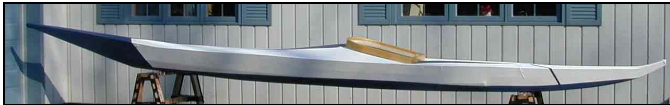
Figure 102. Finished kayak - elevation. Kayak is 22' long, 28 1/2" wide and weighs 61 lbs.
