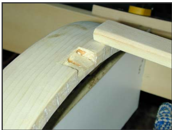
Figure 36. Mortise in masik and deck stringer.
