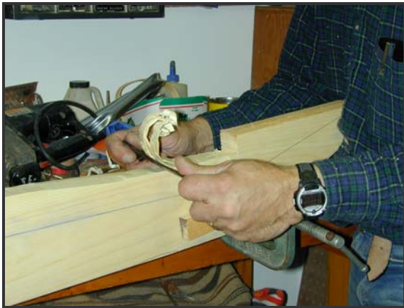
Figure 5. Using drawknife to shape stern handhold.
