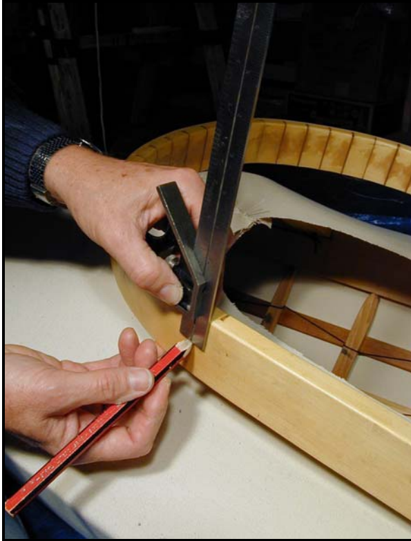
Figure 89. Measuring the coaming for holes 1" below the rim.
