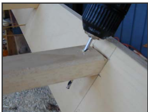
Figure 31. Drilling horizontal hole in gunwale for deck beam lashing.
