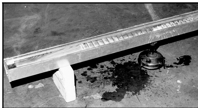
Figure 71. Eaves trough capped on ends for steaming cockpit.
