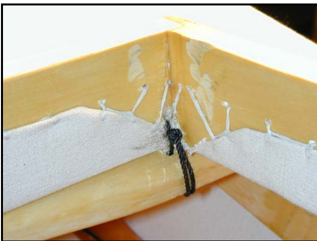
Figure 93. Black seine twine cockpit tied to deck beam.
