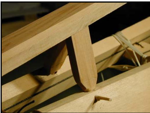
Figure 54. Rib pinned to gunwale.
