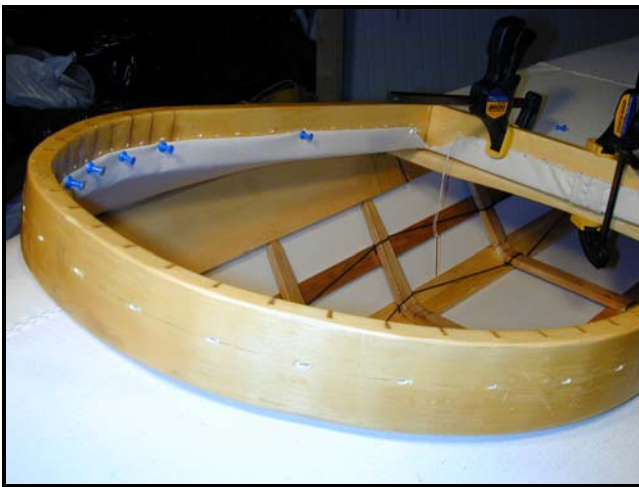
Figure 92. Push pins through canvas in the cockpit coaming.
