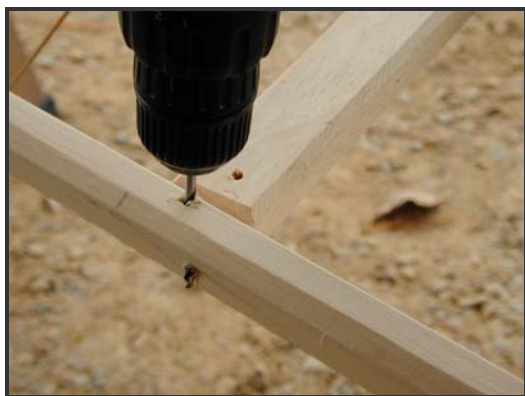
Figure 30. Drilling vertical hole in gunwale for deck beam lashing.
