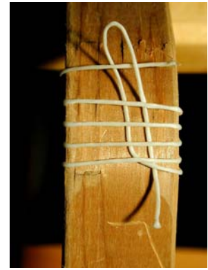
Figure 51. A simple rope whipping.
