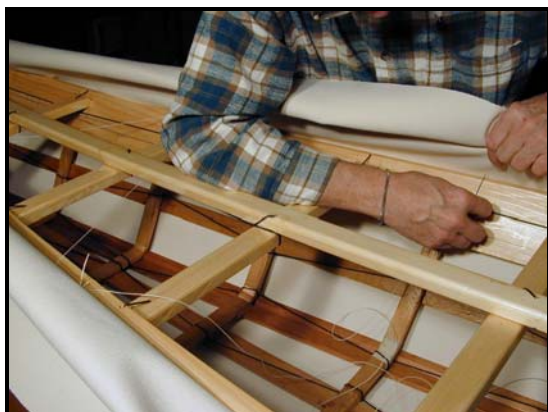
Figure 80. Basting with waxed sailmaker's thread.
