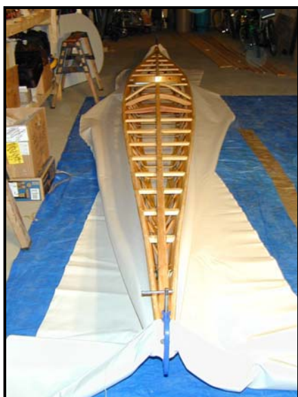
Figure 78. Clamping the canvas bow and stern.
