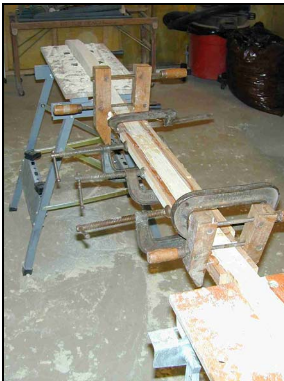
Figure 108. Extra pieces glued to the loom.
