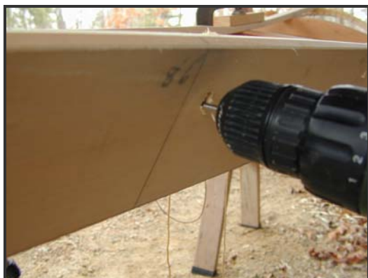
Figure 31. Drilling horizontal hole in gunwale for deck beam lashing.
