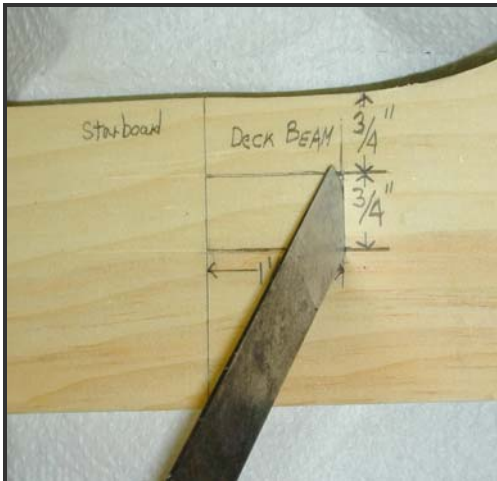
Figure 15. Preparing deck beam mortise in gunwale with chisel at right.
