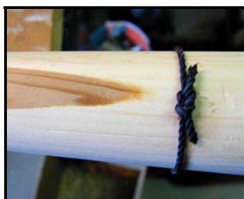
Figure 112. Attach drip rings to paddle. A piece of twine tied with a square knot works well.
