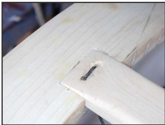
Figure 39. Masik and forward deck stringer lashing.
