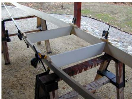
Figure 21. Gunwales spread apart with temporary masik and itivik .
