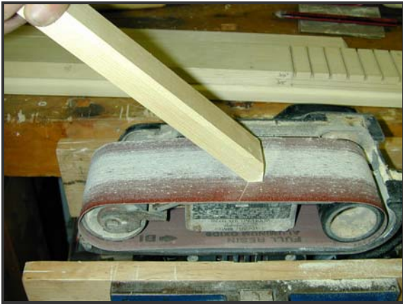
Figure 25. Deck beam on belt sander preparing tenons.
