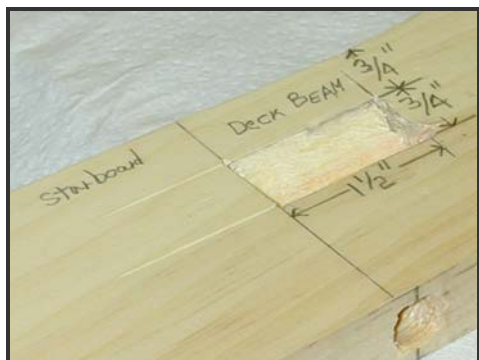
Figure 17. Deck beam finished mortise in gunwale.
