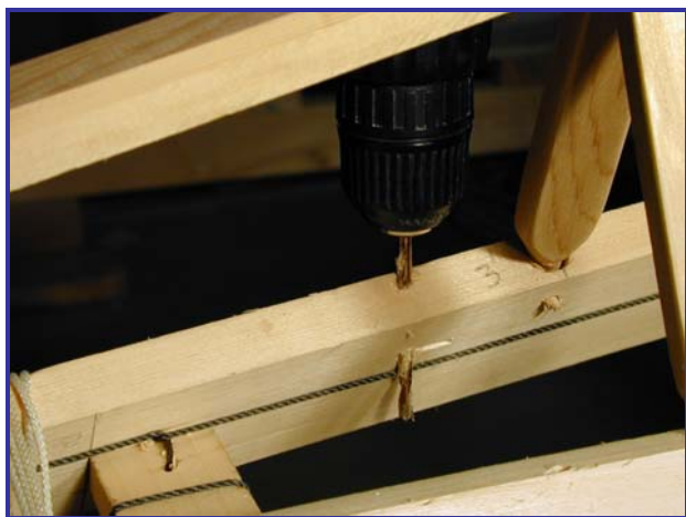
Figure 60. 3/16" hole drilled through the gunwale.
