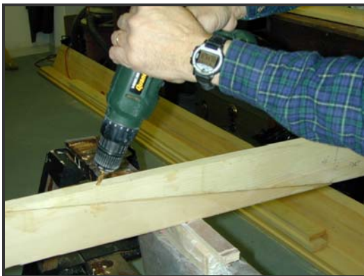
Figure 8. Drilling for wooden pegs in gunwale scarf joint.
